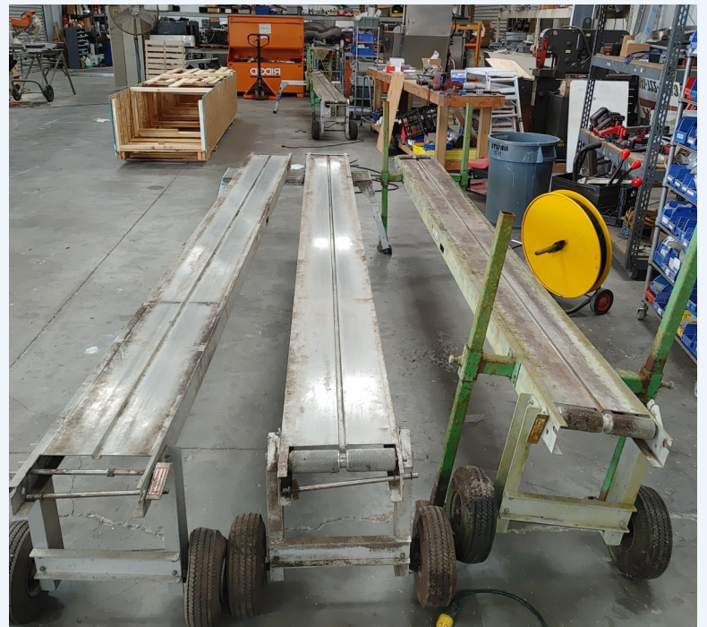
REFURBISHING 25 YR. OLD ADD-A-VEYOR USED IN THE FIELD
