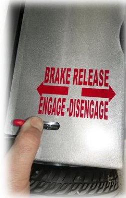
Freewheel feature allows rolling when powered down
