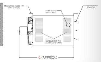
Ratings shown are for elevations up to 2,000 ft. For elevations above 2,000 feet, ratings should be reduced at the rate of 4% for each 1,000 feet above sea level. (In Canada see rating plate) Reduction of rating requires use of a high altitude kit.
